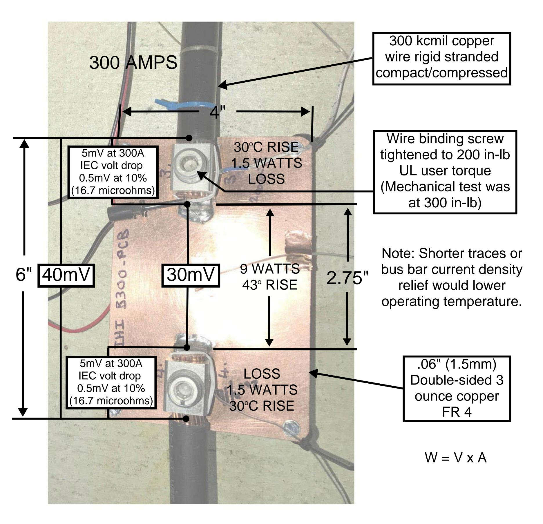
Heat Rise Test B300-PCB using minimal off the shelf FR 4 300 AMP copper wire test current in use rating 285A
